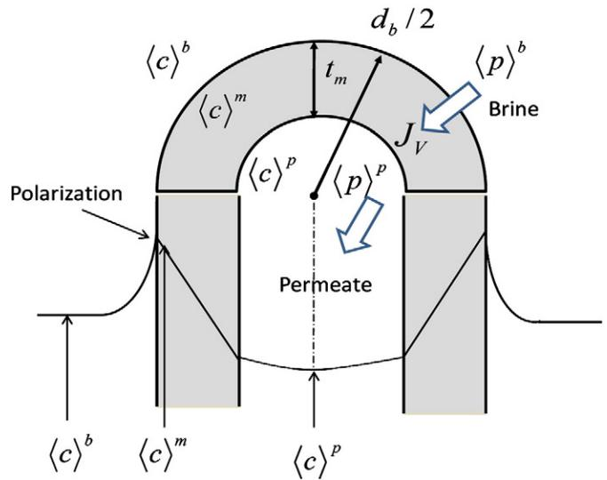
Fig. 2. Concentration polarization in the membrane surface.
