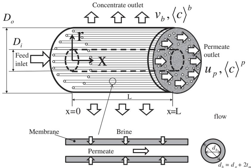
Fig. 1. Radial flow hollow fiber reverse osmosis module.
