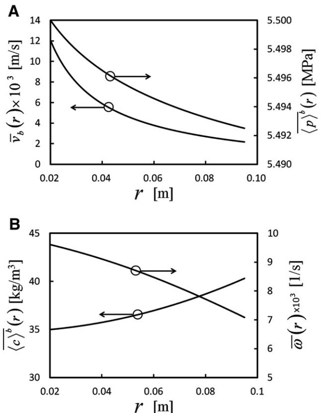
Fig. 6. Radial variations of brine variables. ( $\sigma=0.9$ ,  $Q_{feed} = 15 \times 10^{-4}$  m<sup>3</sup>/s,  $c_{feed} = 35$  kg/m<sup>3</sup>,  $p_{feed} = 5.5$  MPa). (a) Velocity and pressure (b) Concentration and permeate production rate per unit volume.
