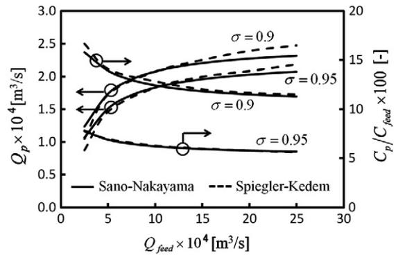
Fig. 5. Variations of permeate variables with feed brine flow rate.
