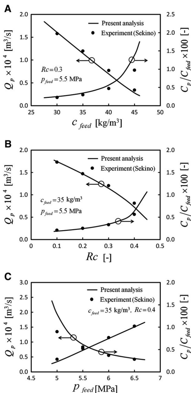
**Fig. 7.** Comparison between the present analysis and Sekino's experimental data. (a) Effects of  $c_{feed}$  on  $Q_p$  and  $C_p/C_{feed}$ . (b) Effects of  $Rc$  on  $Q_p$  and  $C_p/C_{feed}$ . (c) Effects of  $p_{feed}$  on  $Q_p$  and  $C_p/C_{feed}$ .
