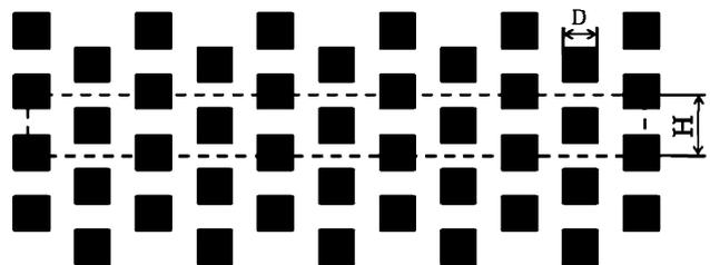
Fig. 4 Physical model for pore scale numerical simulations
